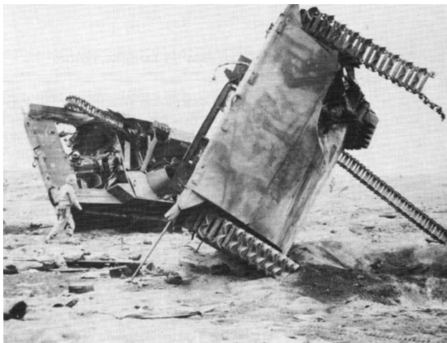
On Iwo Jima, Japanese laid "yardstick" mines on top of aerial bombs. If detonated, the explosions were powerful enough to lift 30 tons of LVT and cargo and blow a hole in the vehicle's bottom.
