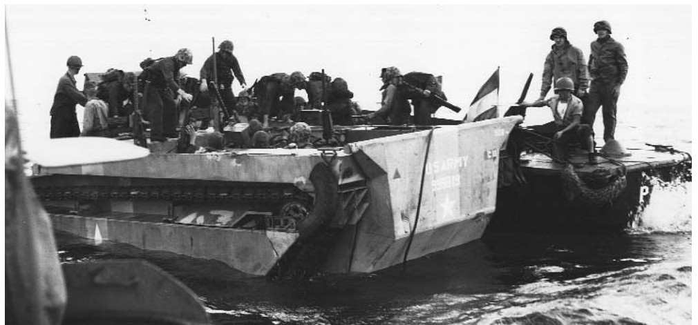
Marine reserves transfer from LCVP to LVT(4) 1,500 yards offshore at Saipan on D-day. The LVT(4), a variant of the LVT(2), had its engine moved forward to permit installation of a stern ramp. It could carry up to 30 troops and as much as 9,000 pounds of cargo, including a jeep or 105mm howitzer. A total of 8,348 LVT(4)s were built during the war.
