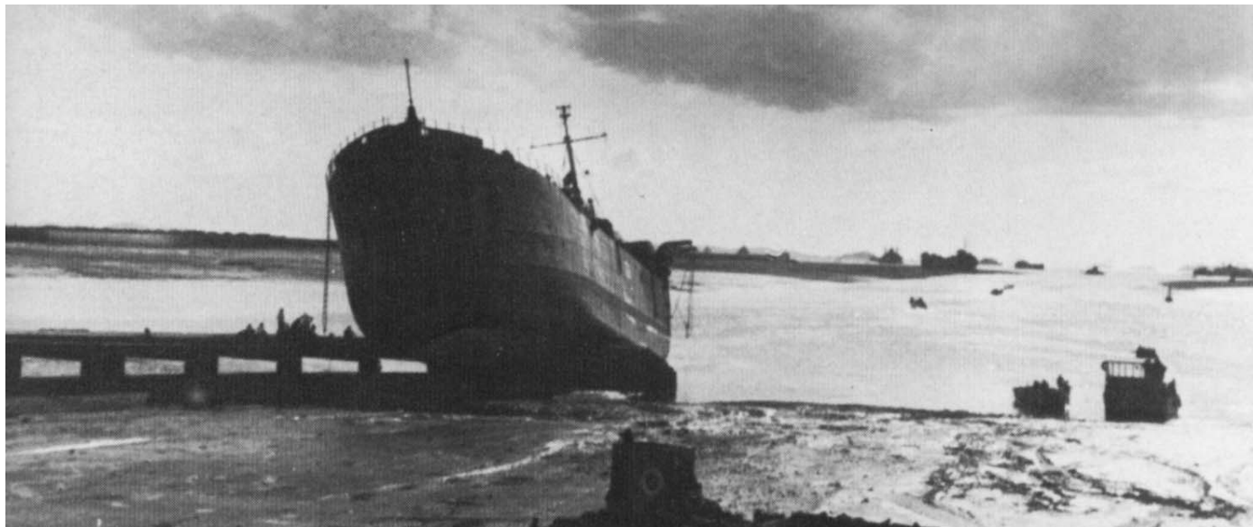
Low tide at Inchon. Tidal range exceeding 30 feet required scheduling main landings at Inchon in early morning and late afternoon.
