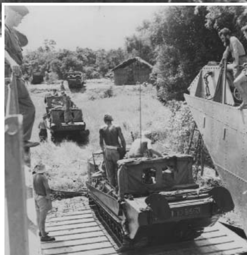
Indochina 1949 M29C (crabs) of 1st Cavalry Regiment of the French Foreign Legion deployed to operational area aboard French Navy Landing Craft. French Archives Photo
