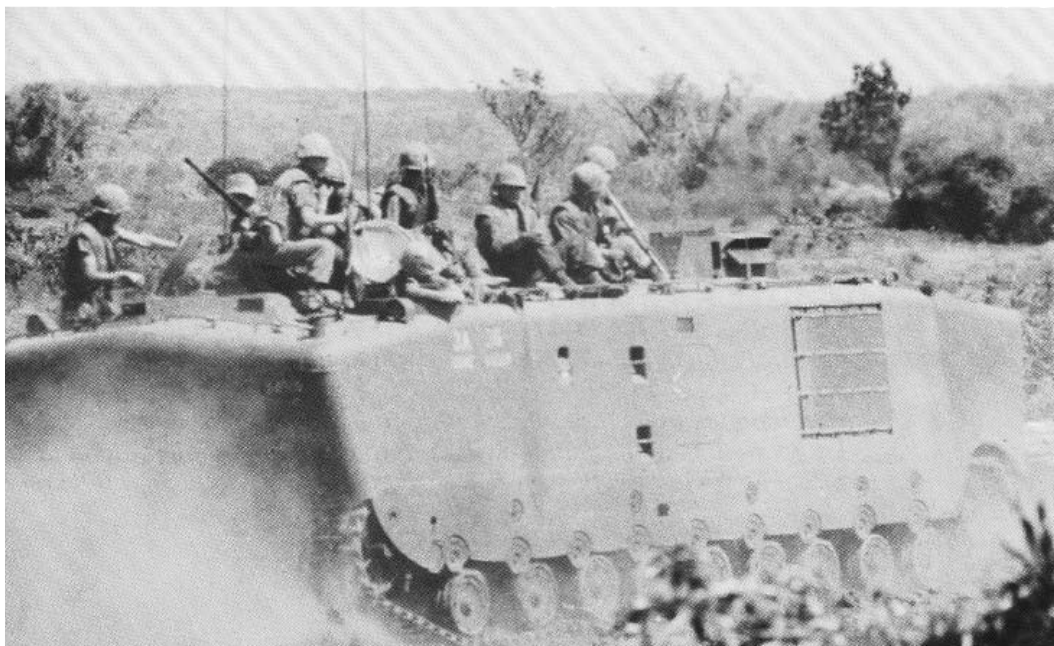
An LVT(P)5 carries its patrol atop the overhead cover in order to minimize any loss should a mine ignite the fuel cells in the bottom of the amtrac. (USMC)
