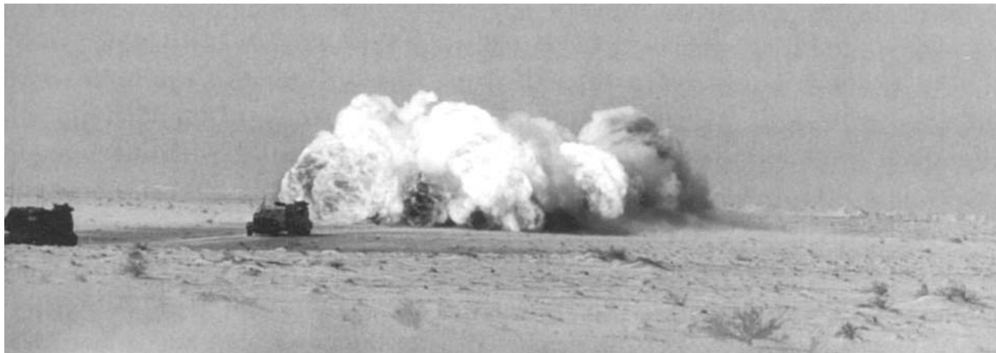
In an early rehearsal for the assault on Iraqi forces in Kuwait, Marines of "Task Force Breach Alpha" fire mine-clearing line charges from special trailers towed by AAV7A1 vehicles. The explosions clear vehicle-wide lanes by detonating, disabling, or moving the mines.
