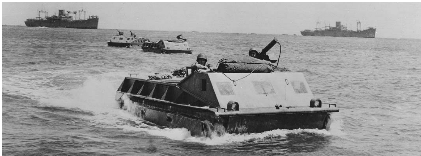
LVT(1)s of the 1st Amphibian Tractor Battalion bringing supplies ashore during the landing on Guadalcanal, 7 August 1942. Note World War I model water-cooled .30 caliber machinegun. Note also canvas cover used to cover cargo compartment in high surf. The LVT(1)s were completely unarmored and were armed with three .30 caliber and one .50 caliber machineguns.
