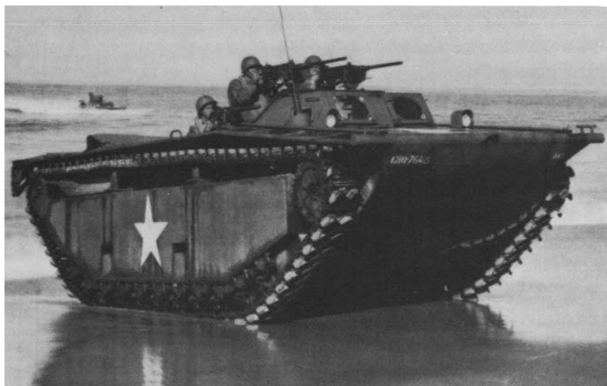
A standard LVT(2), the successor to Roebing's LVT(1). It was the basic design for all amtrac models during WWII except for LVT(3). The LVT(A)2 was an LVT(2) built of armor; the LVT(A)1 was an LVT(A)2 with a 37mm gun turret.
