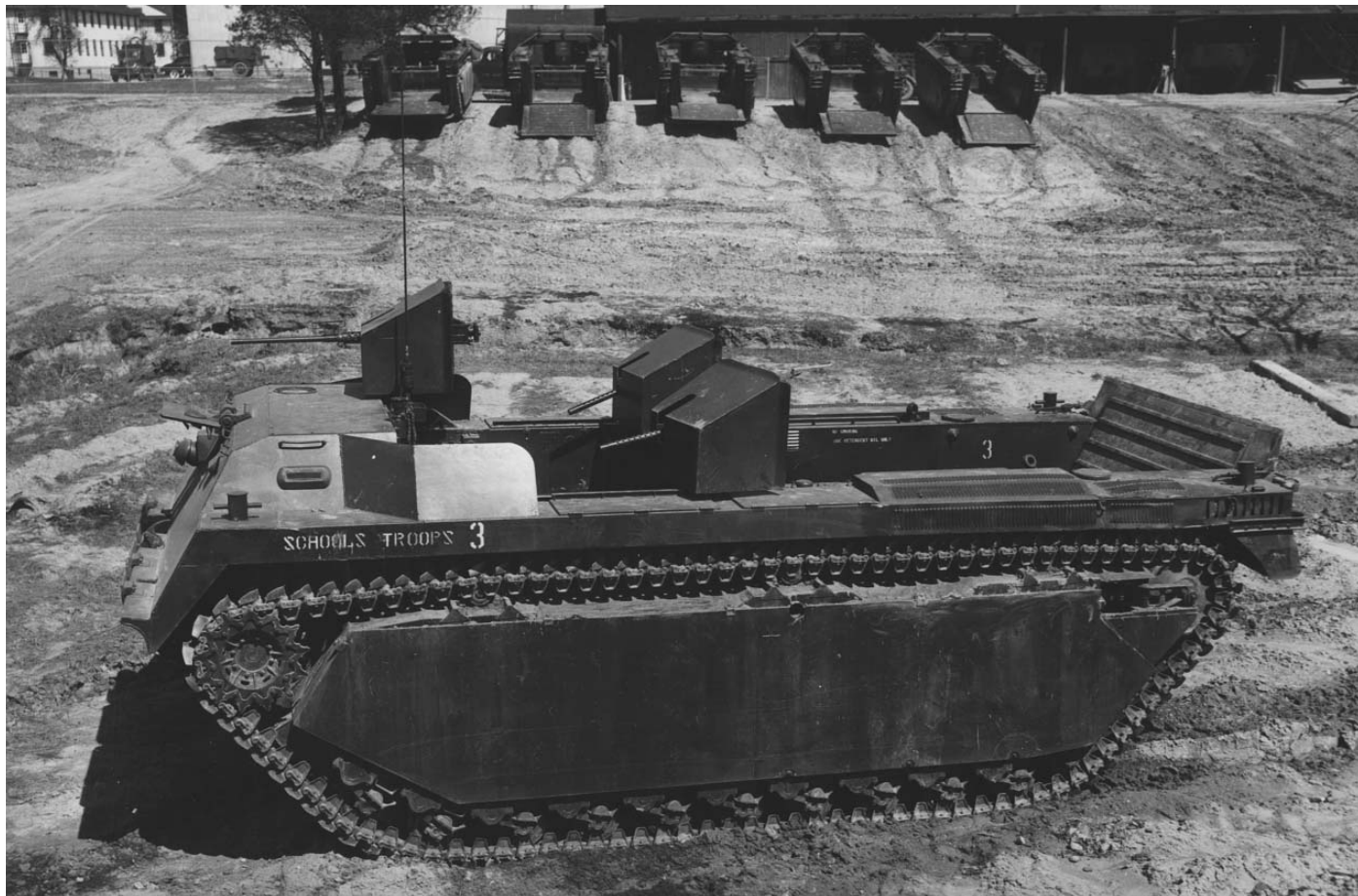
LVT(3)s in use at Quantico in 1950. LVT(3)s were first used at Okinawa. Cargo Capacity: 12,000 pounds, 25% more than LVT(4). Speed: 17mph on land, 6mph in the water. Range: 150 miles on land, 75 miles in water.
